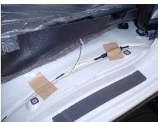
Note: Before securing any of the harness makes sure it is routed to meet the length requirement to make each connection
