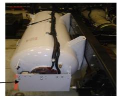
Remove cover plate and set aside (save mounting hardware)
