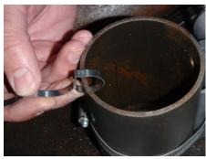
1. Attach pump clip to filter cup
