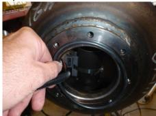
2. Insert rubber o-ring into LPDM flange
