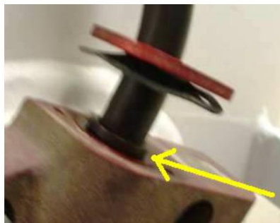
WRONG – LOCKING RING EXPOSED!
