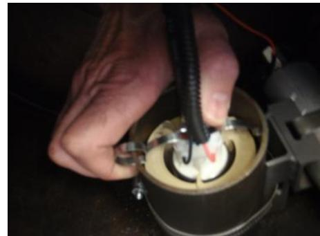
3. Insert the pump from the LPDM into filter cup. Position the pump in cup so the clip goes between the hose and the wires on the pump. Attach the spring to other side of the cup
