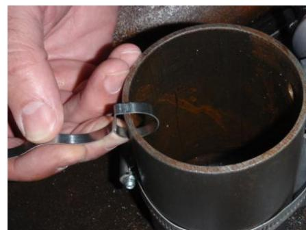
1. Attach pump clip to filter cup
