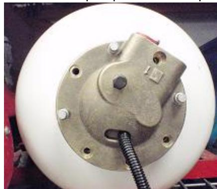
4. Proceed to mounting and tighten LPDM to tank flange. Make sure all hoses and wiring is pushed inside the tank with no kinks or sharp bends. LPDM is clock at 11:00 position.
