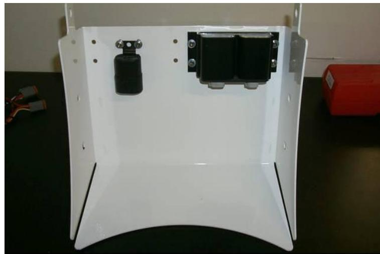
1. Place the Purge Box in alignment over the four holes on the top right corner of the plate. Place the Relay in alignment over the 2 holes in the top left area of the plate. Put washers on all of the screws then place the screws with washers in all four holes in the purge box and two screws in the relay on the front side of the Purge Box and Relay On the backside of the Plate place a nut on each screw and tighten the nuts with your fingers
