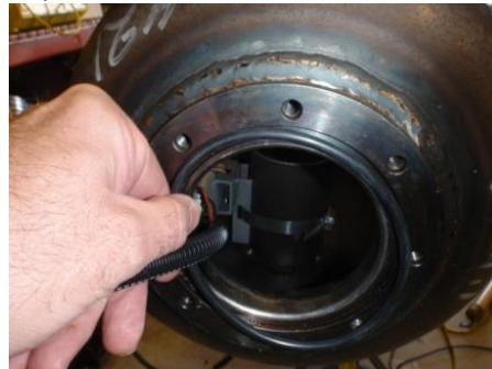
2. Insert rubber o-ring into LPDM flange
