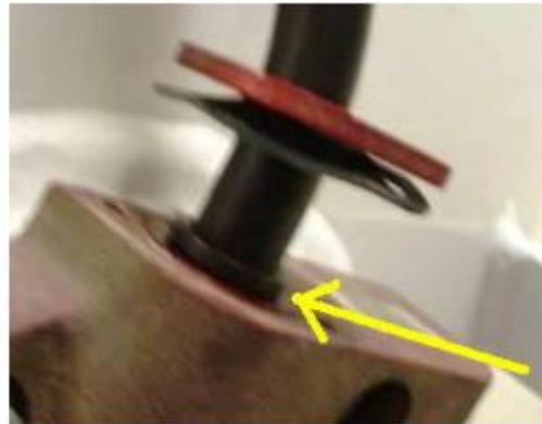
WRONG – LOCKING RING EXPOSED!
